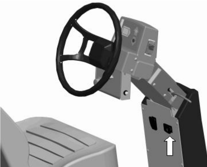
Location of Side Shift Switch
